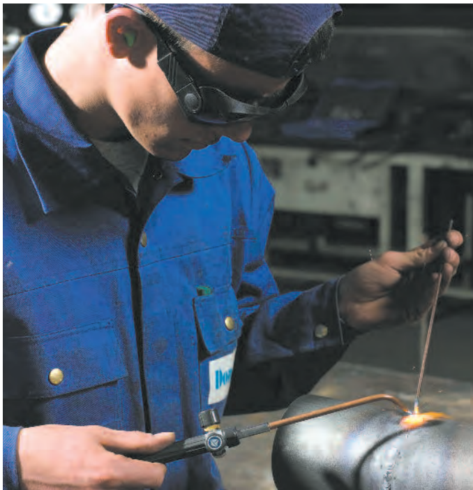
Gas welding on pipes up to material thickness of 4,0 mm
